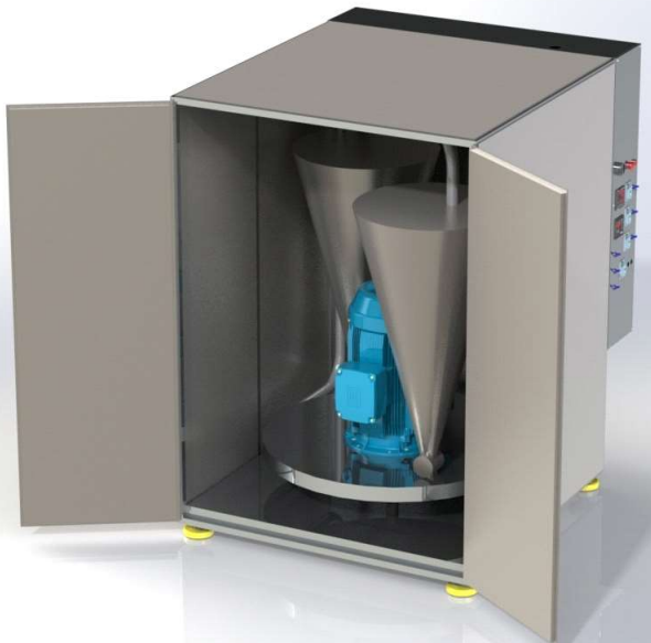
Overall dimensions of the VCU unit: width 1.5 m length 2.0 m height 1.8 m
